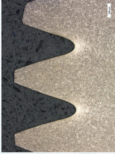
Stainless Steel fastener, external electrolytic etching with 10% aqueous oxalic acid, BF, 50x
