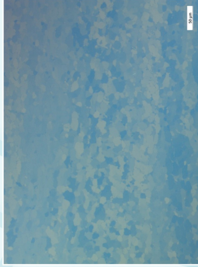
Pure Titanium, Grade 2, POL + Lambda Compensator, 200x
