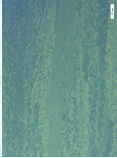
Pure Titanium, Grade 2, POL + Lambda Compensator, 100x
