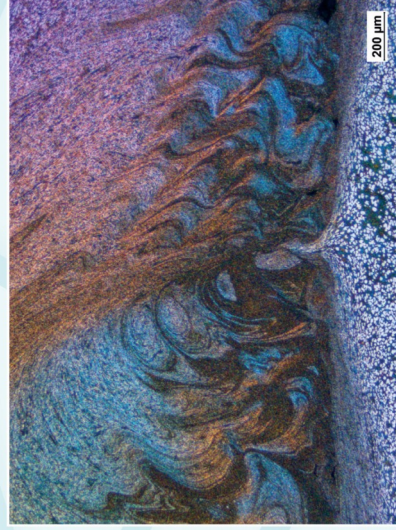
Aluminium friction stir weld, etched according to Barker, POL + Lambda Compensator, 50x
