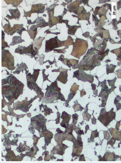
0.45% C Steel, normalised, 200 HV, cross section etched with Nital 3%, BF, 500x
