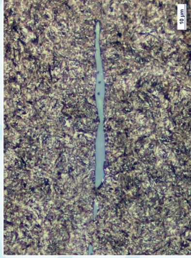
Tool Steel 100MnCrW4+QT, 700 HV, longitudinal section etched with Nital 3%, BF, 1000x
