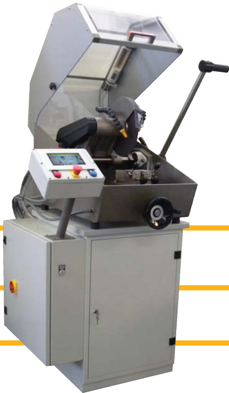
TR 80 with longitudinal table and PLC controlled
